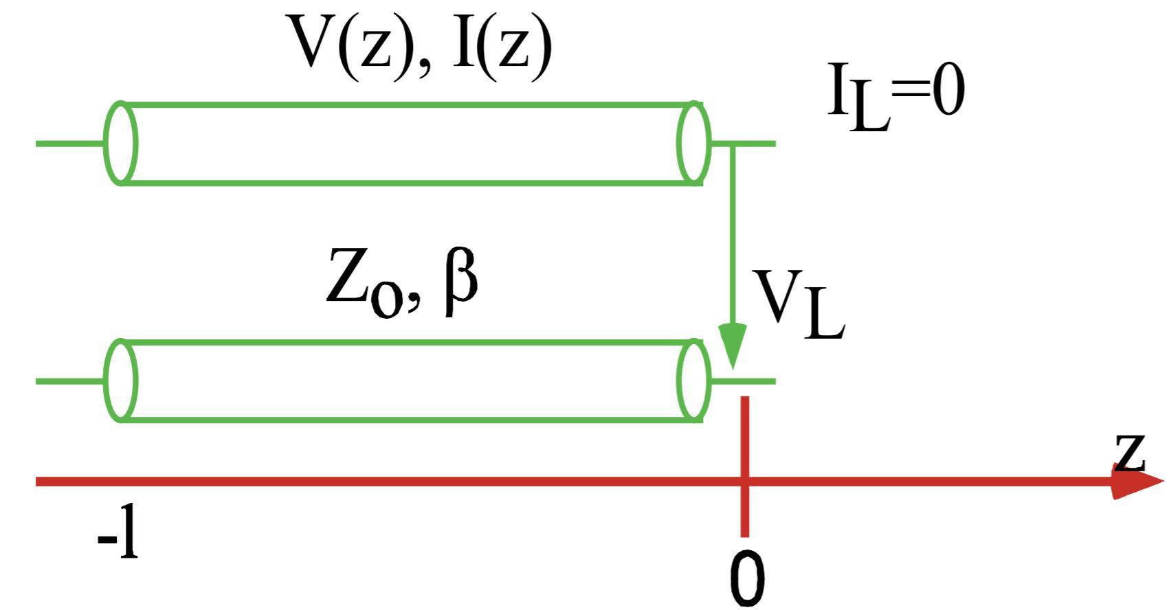
$$V(z) = V_0^+ \left( e^{-j\beta z} + e^{j\beta z} \right) = 2V_0^+ \cos \beta z$$
